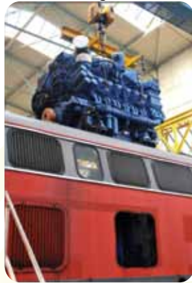
Integration of the MTU prototype engine into the Type 225 008-2 locomotive at the DB AG workshop in Bremen in April 2011.
